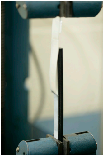
Example of a sample prepared to measure peel force.
